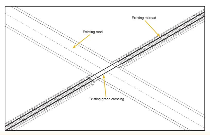
**Goal:** To separate the grades by constructing a multi-span rail bridge and an underpassing roadway.
