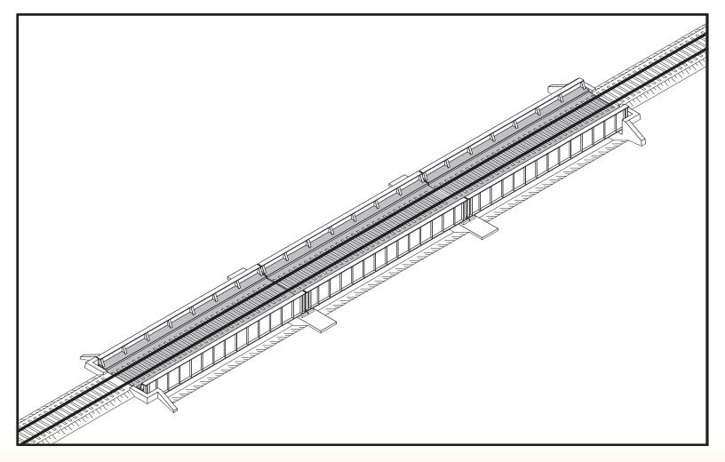
The final bridge span is lifted into place in the same way as the first two. The tracks are connected and the rail bridge is now permanently opened.
