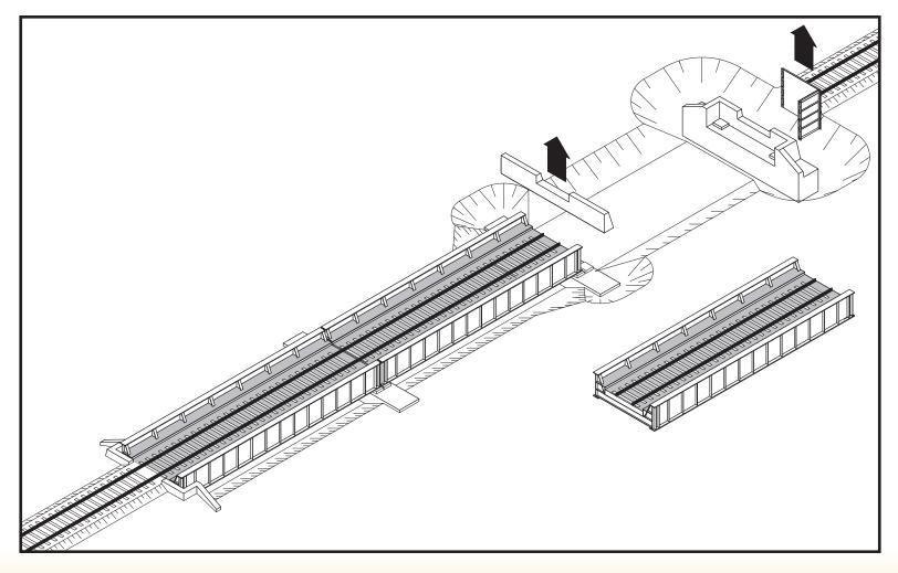
The track is closed for a final four hour period to allow for the placement of the final bridge span.
