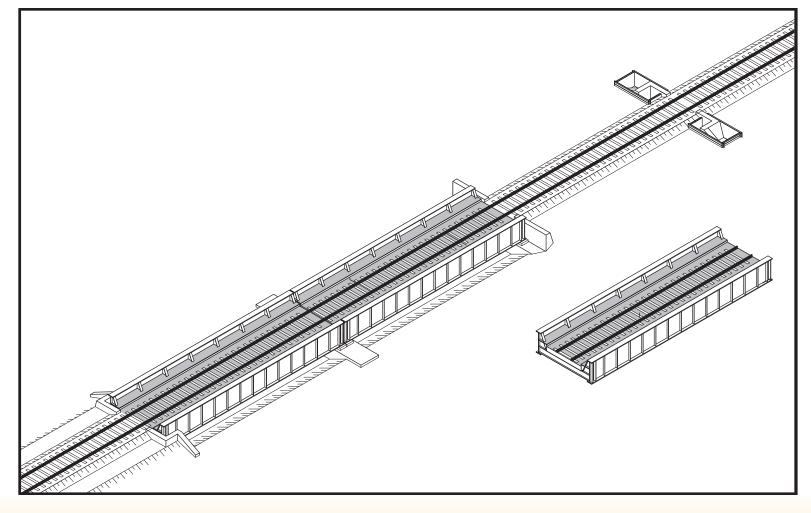
The second bridge span is then lifted into place in the same way as the first to sit on the bearing pads. The tracks are then connected and the railway can be re-opened.
