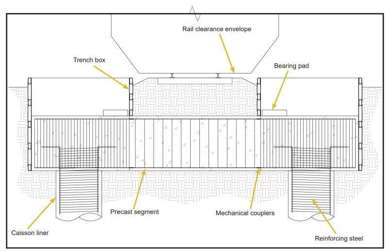
The caisson liners are cut off at the designed elevation and work continues within the trench boxes. The railroad can continue to operate at full capacity as work is performed outside of the rail clearance envelope.
