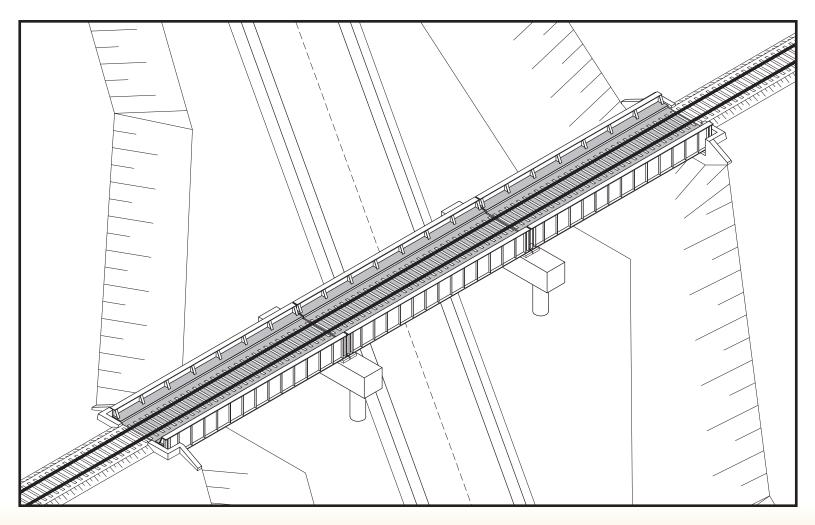
All that is left to do is excavate beneath the track to reveal the completed multi-span rail bridge, install slope paving, and construct the under-passing roadway.
