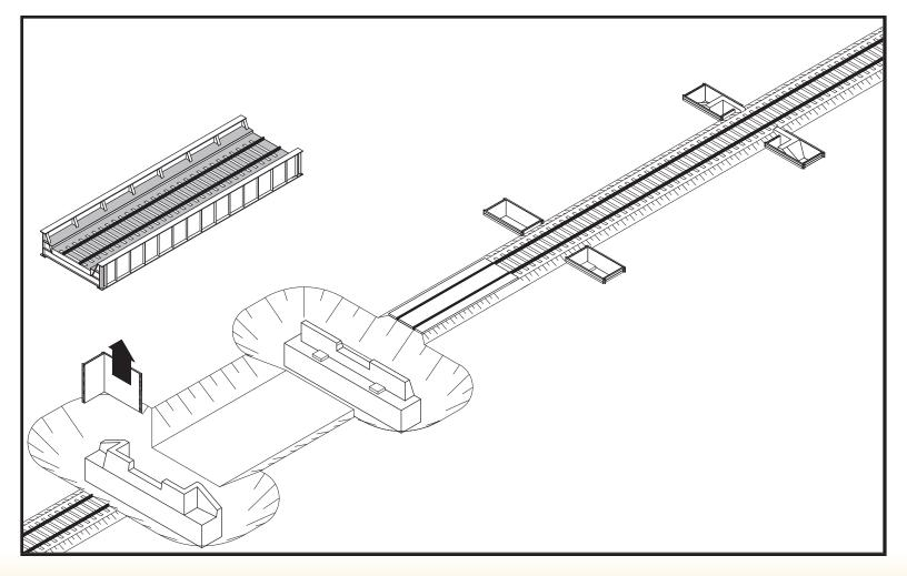
The track is closed for a second four hour period and a trench is dug between the first abutment and pier cap. The trench boxes are then removed. These trench boxes are reusable to help cut down on wasted material.
