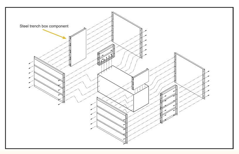
Steel GSS trench boxes are bolted directly to the precast substructure segments with threaded rods or bolts.
