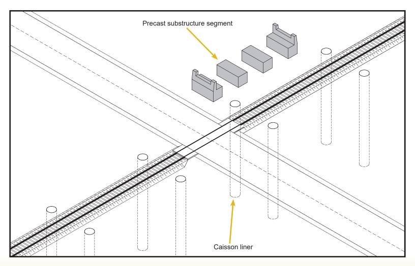
Caisson liners are installed outside of the rail clearance envelope, a minimum of 9 ft away from the centre line of the track.
