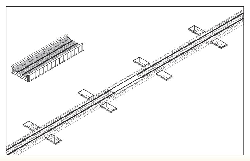
While work continues within the trench boxes, the bridge span(s) are assembled to the side of the track.
