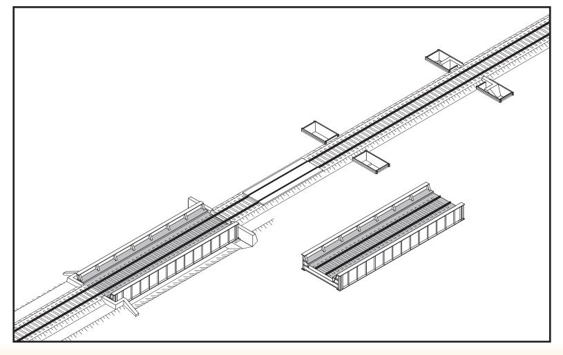
The completed bridge span is then lifted into place to sit on the bearing pads. The span can be lifted with two 300 ton cranes or a lateral slide. A temporary ballast wall can be used at the pier cap if required. The tracks are then connected and the railway can be re-opened.
