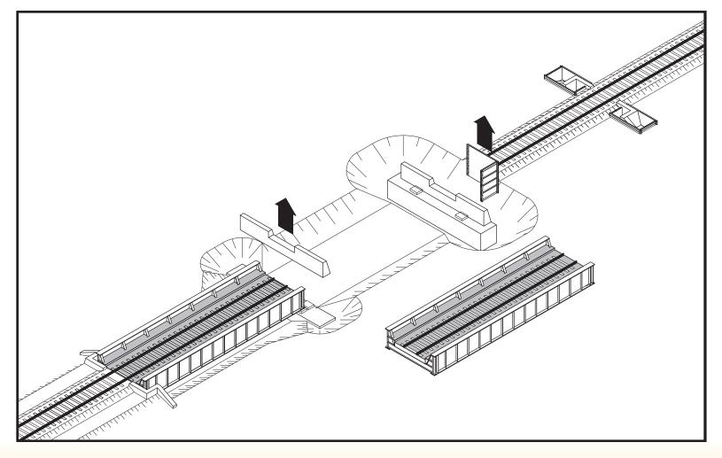
The track is closed for another four hour period to allow for the installation of the second bridge span. A trench is dug between the two pier caps and the trench boxes are again removed.
