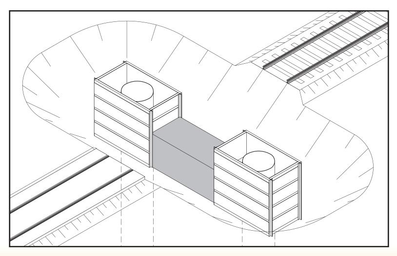
The track is closed for a four hour period and a trench is dug across the tracks. Most rail companies can easily accommodate overnight for this closure period.
